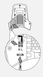
Connecting to an installed socket next to or behind the appliance
